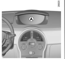
**The instrument panel A** lights up when the ignition is switched on. In some cases, the appearance of a warning light is accompanied by a message.
