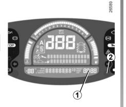
The time is displayed when the ignition is switched on.
