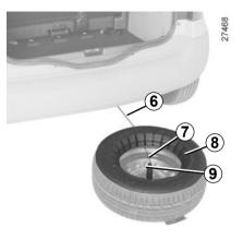
After changing a wheel, position the replaced wheel on support 9, with the valve facing the ground. Depending on the vehicle, reposition shim 8. Clip cable 6 into housing 7, then push the wheel underneath the luggage compartment (tab 10 towards the rear of the vehicle).
