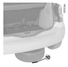
Position yourself behind the vehicle and pull handle  $\boldsymbol{5}$  to raise the wheel until it is anchored under the vehicle.
