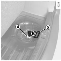
unscrew nut 4 in an anti-clockwise direction until it comes off completely, then place the palm of your hand on section B of handle 5 and push towards the front of the vehicle. The wheel will be lowered.
