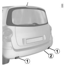
On vehicles equipped this accessory, the rear bumper is fitted with two flaps covering the mounting points for the bike rack and an electrical socket **2** located underneath the vehicle.
