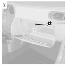
Depending on the vehicle, this glove box compartment is ventilated and air conditioned in the same way as the passenger compartment.
