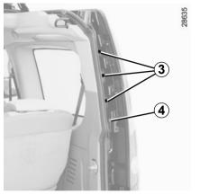
unscrew the screws 3 and remove cover 4;
