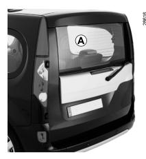
The permissible load on the tailgate with the window lowered is 50 kg.
