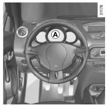
**Instrument panel A**: you can adjust the brightness from the trip computer and warning system.
