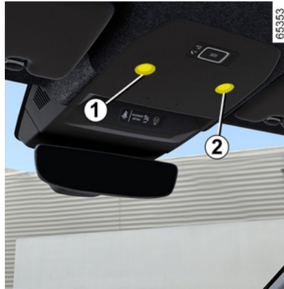
Reading lights 1 and 2
