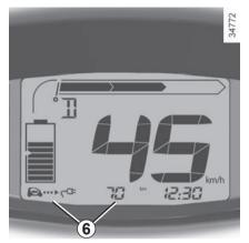
Zones **6** of the instrument panel display the information detailed below by pressing button **5** repeatedly:
