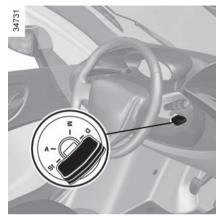
Before towing, insert the key in the switch to unlock the steering column. Turn key to position  $\mathbf{M}$ .
